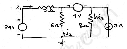
b) For the circuit shown below, find the potential difference between a and d:
