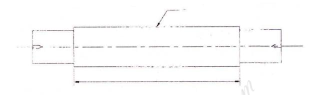
Material – M.S. Rod 25 mm dia. 265 mm length.
