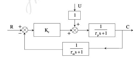
A unit step input is introduced in the set point. The value of  $K_c$  to provide a critically damped response for U = 0,  $\tau_{\rm p}$  = 8 and  $\tau_{\rm m}$  = 1 is
