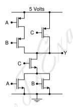
(A)  $Y = \overline{A}\overline{B} + \overline{C}$
