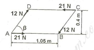
Determine the angle  $\beta$  if the resultant couple is 1.8 N.m clockwise.
