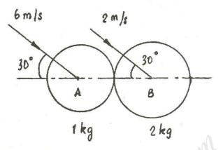
If the coefficient of restitution is 0.5, find the velocity and the direction of the two balls after impact. Also calculate the loss in kinetic energy due to impact and the percentage of loss. (16)
