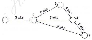
Determine the Project duration, Locate the Critical Path and CRASH the network by 4 wks and find out the total cost.
